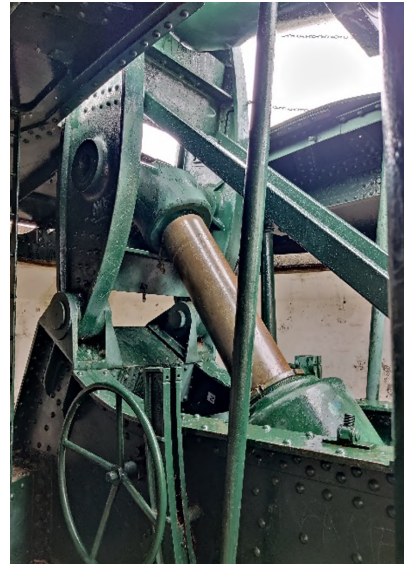
Above- Gun recoil mechanism
