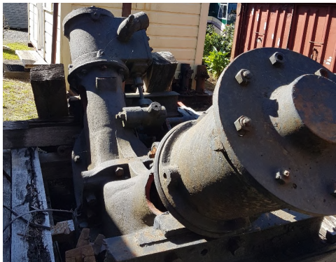
Above: The V-Twin cylinder configuration. Heisler.
