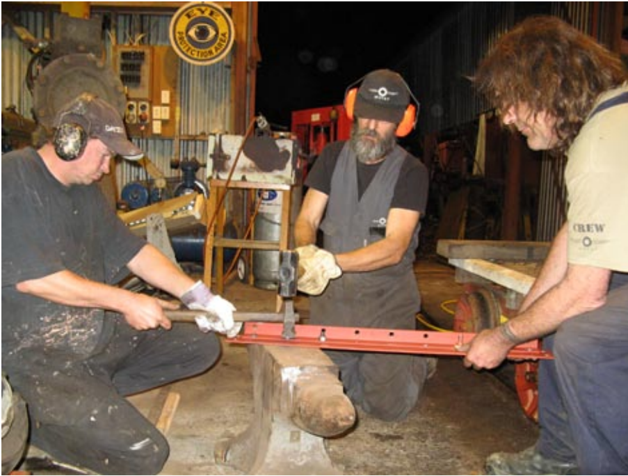
LEFT: Andrew Holembly holds a die block, as Paul Spearpoint, wields a sledgehammer to shape the red hot rivet, with Ted Leach holding the metal bars which were to form part of the rear cab panel on April 29 2009. Nuts and bolts held everything in place, until being replaced by the rivets.
