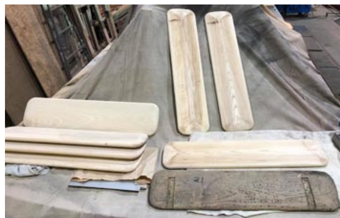
The American Ash seat backs ready for the seat stanchion rebates to be machined in. These were manufactured by Styrotech to a CNC program supplied by Leyton Chan and finished in the tram workshop. An original which was used as a pattern is in the foreground.
