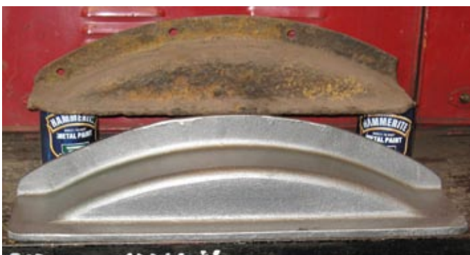
New coal bunker splashers arrived from Progressive Castings of Avondale, shown here with an old one. These were cast to patterns made by Paul Spearpoint.
