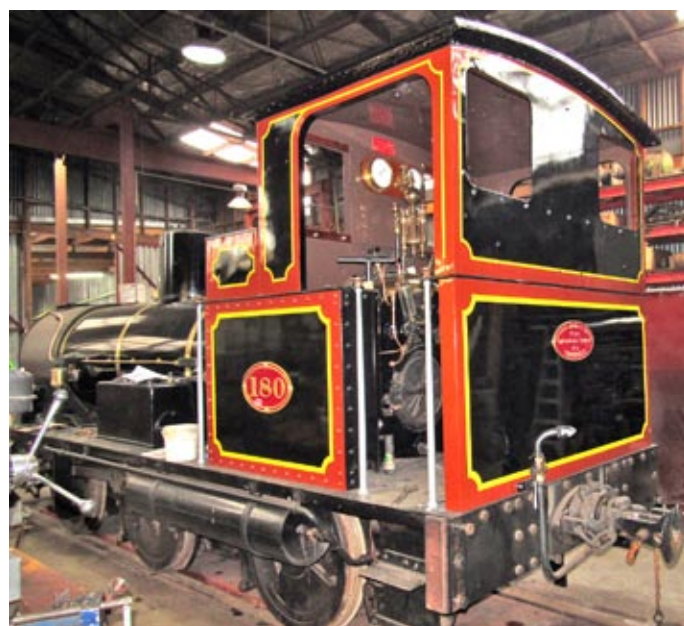
In 2016 it was the turn of painter signwriter Shane Price to work his magic on Meg. LEFT on February 21 Meg had received its coat of black, and BELOW on July 17 it was resplendent in its fully lined 1909 colour scheme of black and Indian red with yellow lining with its boiler bands polished.
