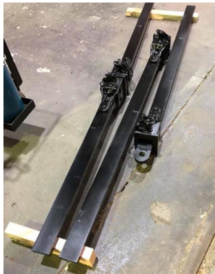
The coupling bars to join trailer 21 to steam tram 100 after their arrival from the manufacturer. Left are the two parts joined, while right are the parts separated.
