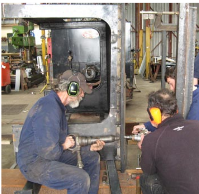
Six years later and it was turn of the top panels of Meg's cab to be hot rivetted together. On July 5 2015, Paul Spearpoint is pictured with Murray Wilson during a special public demonstration day organised by the museum
