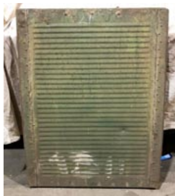
ABOVE LEFT: One of 21's original corrugated aluminium wall panels with post service garden shed green paint.
