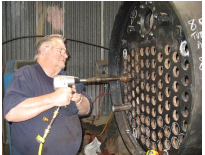
Boiler work was also underway as Jim Savage is shown honing the tube plate for the tubes on April 14 2009.
