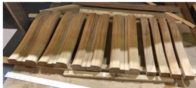
The four bulkhead end seat backs and their stiffeners ready to be assembled with the light and dark seat slats.
