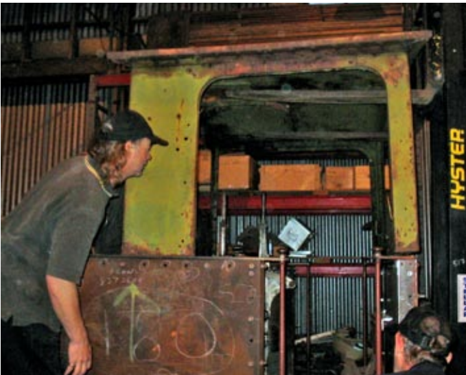
March 11 2009 the sheet metal work for the cab rear and the bunker sides was underway and a trial fitting was held with the top part of the old cab, seen here with Stuart Capon checking the fit. This was then dismantled for the finishing work. It would be 2015 before the cab would be finally assembled.
